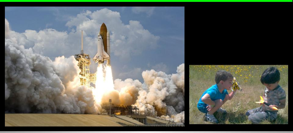
Equal and Opposite: The downward force of the rocket fuel is opposite to the upward force on the rocket.
