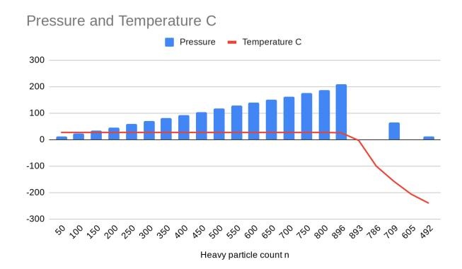
Figure 9. Graph showing that temperature dropped steeply after maximum pressure was exceed. The top of the chamber opened and gas escaped. Pressure reduced to 0.6 atm.
